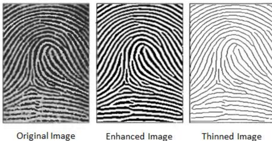
Figure 7. Enhancing and Thinning a Webcam Image,
