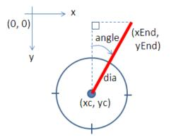
Figure 12. Calculating an End Point.
