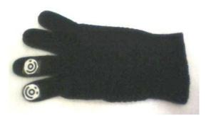
Figure 3. A Glove with Attached TopCodes.
