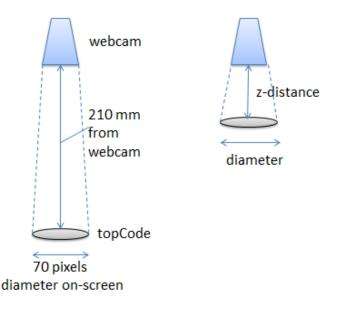
Figure 10. Converting TopCode Diameter to z-distance.
