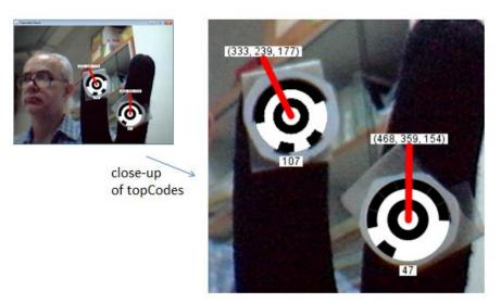
Figure 6. TopCodes Rendering in the Webcam Window.
