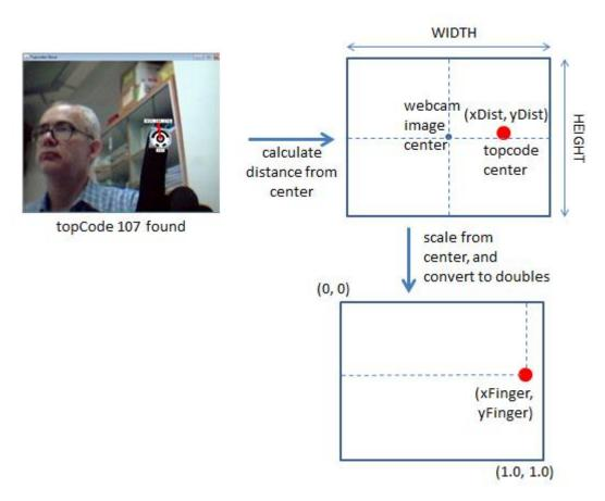
Figure 8. Converting a Finger Coordinate to a Target Position.
