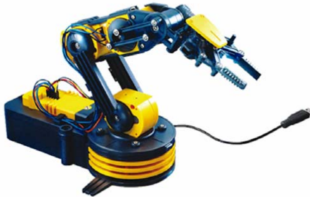
Figure 1. The OWI-535 Robotic Arm with USB Interface.
