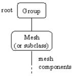
Figure 5. Format of a Scene Graph with a Group Node at its Root.
