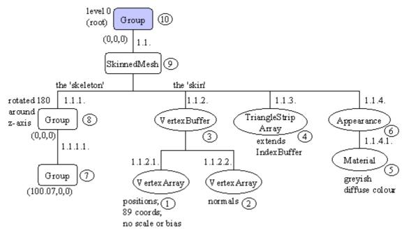
Figure 6. Scene Graph Loaded from tube.m3g.
