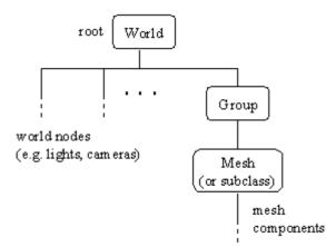
Figure 4. Format of a Scene Graph with a World Node at its Root.
