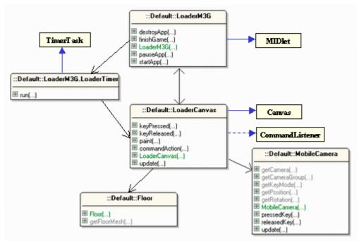
Figure 13. Class Diagrams for LoaderM3G.
