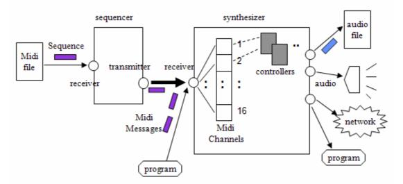
Figure 12. A MIDI Sequencer and Synthesizer.
