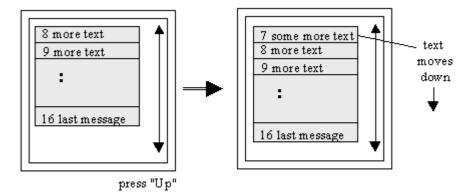
Figure 8. Press "Up" to Move the Messages Down.
