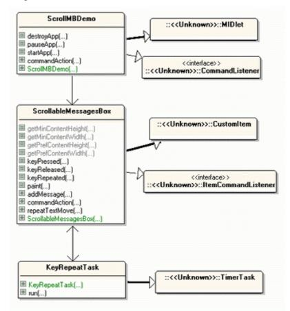
Figure 4. Class Diagrams for ScrollMBDemo.
