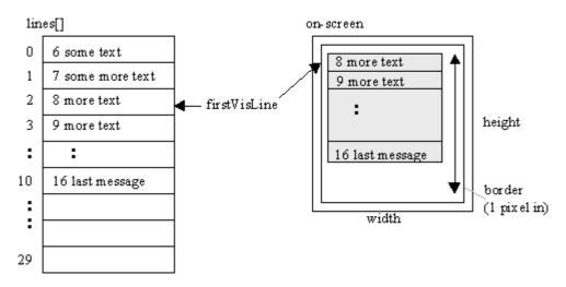
Figure 5. Message Storage and On-screen Appearance.
