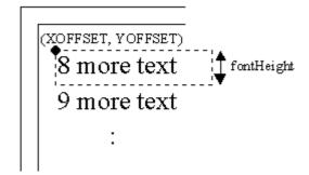
Figure 6. The Drawing Coordinates for the Message Lines.
