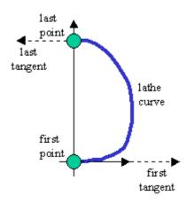
Figure 11. Typical Lathe Curve with Tangents.
