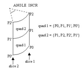
Figure 12 shows how two quads are defined. Each point is stored as three floats.
