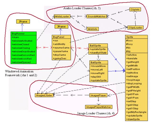
Figure 2. Class Diagrams for BugRunner.
