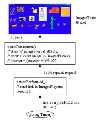
Figure 12. ImagesTests and the Swing Timer.
