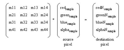
Figure 22. BandCombineOp as a Matrix Operation.
