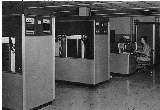
An IBM 305 RAMAC, with two 350 disk drives in the foreground. Photo by US Army Red River Arsenal.
