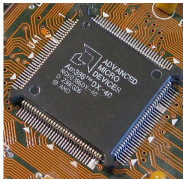
An AMD Am386DX-40 Chip. Photo by MaXim. GPL.
