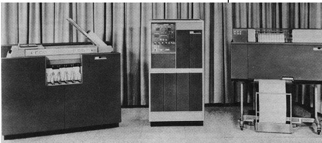
IBM 1401 System. From the left: 1402 Card Read-Punch, 1401 Processing Unit, 1403 Printer (1961). Photo by Gobierno de los Estados Unidos.
