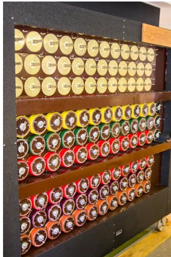
An accurate bombe replica, built by the "Phoenix" team led by John Harper (2008). Photo by Antoine Taveneaux. CC BY-SA 3.0.
