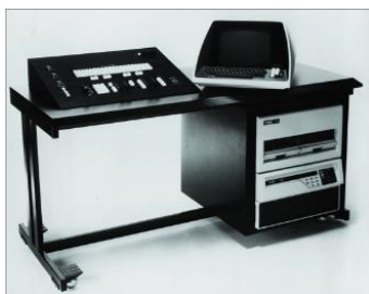
The LS-8 computerized lighting console.
