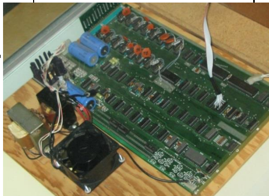
The Circuit Board of a Fully Assembled Apple I. Photo by geni. CC BY-SA 4.0.
