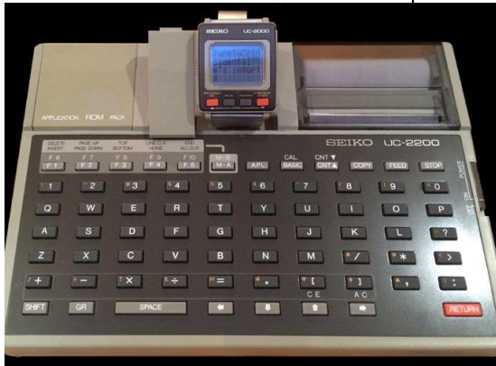
A Seiko UC-2000 (center top) plugged into a UC-2200. Note the thermal printer of the right and ROM pack on the left (1984). (c) Seiko
