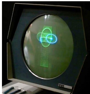
A PDP-1 Type 30 Display running the Minskytron. Photo by Joi Ito. CC BY 2.0.
