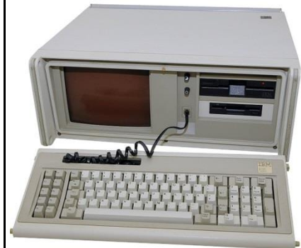
The IBM 5155; the disk drive on the right was installed later. Photo by Hubert Berberich. CC BY-SA 3.0.
