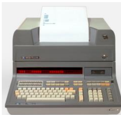
A HP 9830A with an optional 9866 thermal printer mounted on top. Photo by Hydrargyrum. CC BY-SA 3.0.
