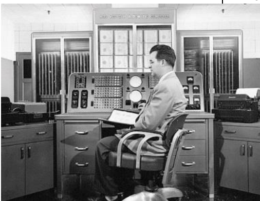
The SWAC, including Williams-Kilburn tubes (center background). National Institute of Standards and Technology.
