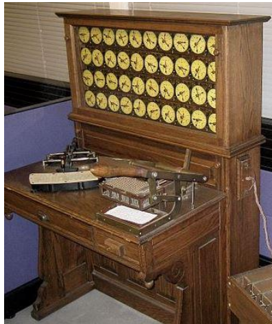
Replica of a 1890 Hollerith tabulating machine. Photo by Adam Schuster. CC BY 2.0.
