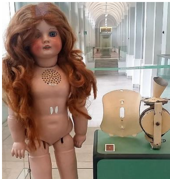
An Edison Phonograph doll, 1890. The mechanism housed in the body has been removed and is displayed alongside. Photo by Mabal. CC BY-SA 4.0.
